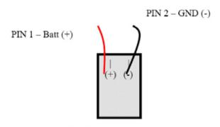
1) Connect the **RED wire** from the Charging wiring harness to pin **19**, "**BATT**" of the respective RTU device. The Master and Slave controllers are identical in wiring, features and programming. Be sure a 1 Amp FAST blow fuse is installed.
